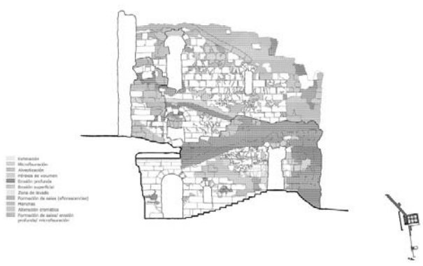
Figure 8 Analysis of the pathologies affecting the materials. Detail of the south face.
